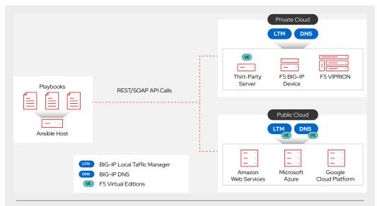
Figure 1. Red Hat Ansible Automation Platform can manage F5 devices in both private and public cloud environments.
